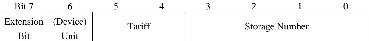
Fig. 22 Coding of the Data Information Field Extension (DIFE)
