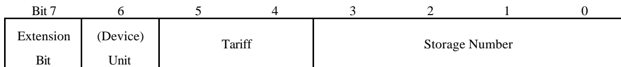
Fig. 5 Coding of the Data Information Field Extension (DIFE)
